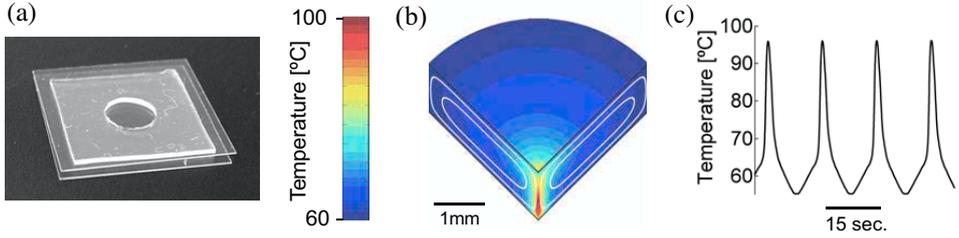
Fig. 5. Toroidal Convective PCR. (a) A cylindrical chamber is centrally heated by infrared radiation.<sup>11,12</sup> (b) This triggers a toroidal convection flow. (c) The calculated temperature along the paths of the flow shows for about 50% of the volume short and high temperature peaks that directly mimic the temperature pattern of standard PCR. The flow speed dispersion is quite low due to the lack of internal boundaries. Figures (b) and (c) reprinted with permission from Refs. 11 and 12.
