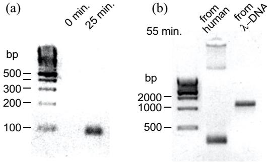
Fig. 6. Results of toroidal convective PCR. (a) A 96 base pair product from  $\lambda$ -DNA shows at least  $100,000 \times$  amplification after 25 minutes.<sup>11</sup> (b) A chamber with half the thickness and twice the radius allows to amplify a 295 base pair sequence from human DNA and can amplify even 1,100 base pair products. Figure (a) reprinted with permission from Ref. 11.
