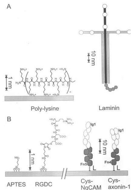
Fig. 1. Dimensions of adhesion molecules immobilized on silicon oxide. (A) Polylysine and laminin were immobilized by physisorption. (B) APTES, RGDC, Cys-axonin-1 and Cys-NgCAM were covalently immobilized on the oxide via silane chemistry with a crosslinker molecule for an oriented immobilization. (L, peptide linker with C-terminal Cys, crosslinker and amino silane; Ig, immunoglobulin-like domain; Fn, fibronectin-like domain).
