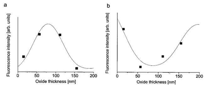
Fig. 4. Determination of minimum and maximum cell–surface distances. The average fluorescence intensities of boxes r1–r4 (a) and R1–R4 (b) of Fig. 2c were plotted vs. the four different oxide thickness (■). The curve was fitted with the distance calculation program (see text). The calculated distances were  $34 \pm 5$  nm for (a) and  $154 \pm 7$  nm for (b).
