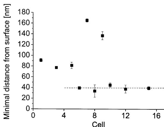
Fig. 6. Calculated minimal distances from all cells measured on RGDC-treated chips. Low values are clustered in a mean cell–substrate distance of 39 nm (dashed line).
