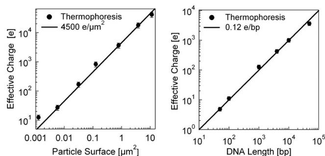
**Fig. 5.** Effective charge from thermodiffusion. Effective charge is inferred from thermodiffusion using Eq. 3. Polystyrene beads (20–2,000 nm) (a) and DNA (50–50,000 bp) (b) were measured over a large size range, which is impossible with electrophoresis. As expected, the effective charge of the beads scales with particle surface and linearly with the length of DNA.
